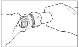
SNAP SNAP THE COUNTERSTRIKE® TUBING INTO THE BACK END OF THE FITTING
