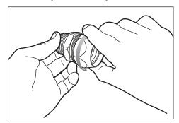
**TWIST** TWIST NUT ONE TO ONE AND A HALF COUNTERCLOCKWISE TURNS
