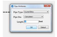
Select the pipe type, usually *CounterStrike*, and specify the length of the pipe in feet. The pipe type will be remembered for next time. Click *OK*. *Pipe Dia*. is for existing pipes in legacy systems or for forcing explicit sizes.
