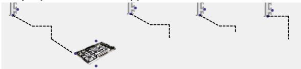
• After you draw a pipe, you can adjust it using the *select* tool. If you move the mouse over a multi-bend pipe, you see middle sections highlight. If a section is highlighted, you can click on it and move it around, horizontally for vertical sections, vertically for horizontal sections, or any direction for *direct* sections—ones at an angle. To move the first or last section of a pipe, move the appliance it is connected to, or its end point.
