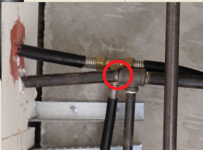
Recent UC San Diego earthquake testing proved that black iron pipe fractured and leaks while the CounterStrike CSST remained leak free.
